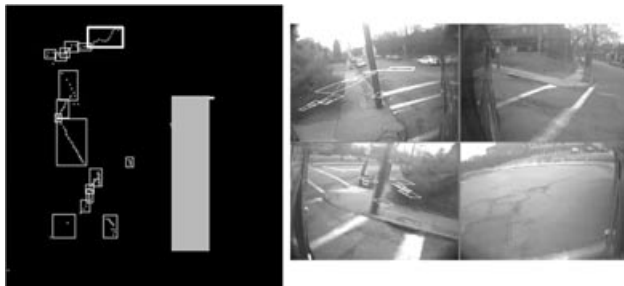
Figure 18. Ground returns seen as an object in the left front of the bus (thick white box).
