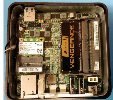
Figure 9: The inside of Phaser AP with one Intel 5300 card shown. Two NICs are employed to have a total of six available RF chains.
