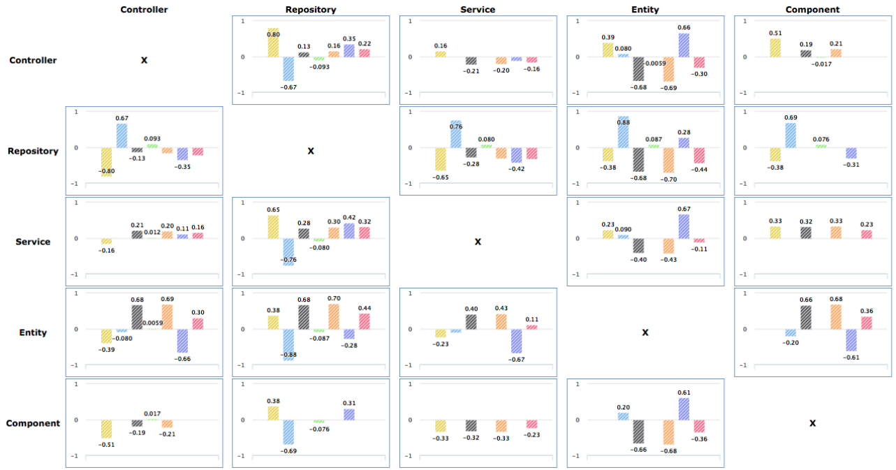
Figure 3: Code metrics distribution in the system (bars, from left to right: Yellow=CBO, Blue=DIT, Black=LCOM, Green=NOC, Orange=NOM, Purple=RFC, Pink=WMC). Striped bars = significant difference ( p\text{-value} < 0.05 ), height = Cliff's Delta effect size.
