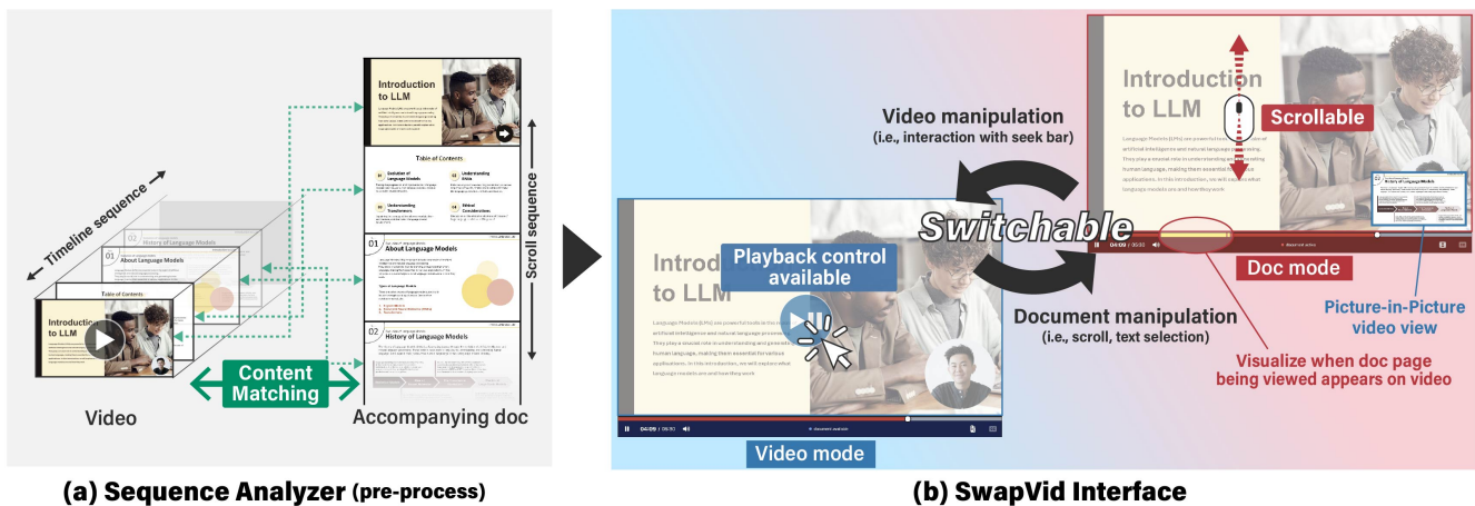
Figure 1: SwapVid is a novel interface that supports document-based video viewing; (a) our sequence analyzer performs content matching between each video frame and the document; (b) based on this, the interface integrates the video viewer and document viewer into a single window and seamlessly switches between them upon the user’s direct manipulation of the video/document.
