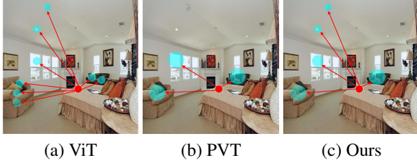
Figure 2. Comparison of different attention mechanisms in Vision Transformer (ViT), Pyramid Vision Transformer (PVT), and our SSA with the same feature map size. The number of circles represents the number of tokens involved in the self-attention computation, and reflects the computation cost. The size of the circle indicates the receptive field size of the corresponding token. Unlike ViT and PVT, our method adaptively merges circles on large objects for enhancing computation efficiency, and accounts for objects of different scales simultaneously.
