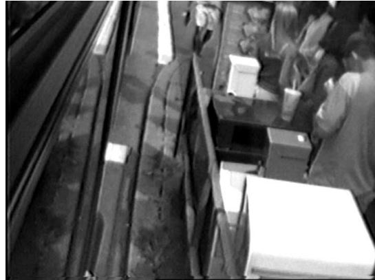
Figure 2 Operating environment of a transit bus. The picture is taken from the top rear right corner of the bus, looking down along the side of the bus, which is visible in the left part of the image. The bus has just left a bus stop and is only one foot away from the curb. Two to three feet away are people and objects.
