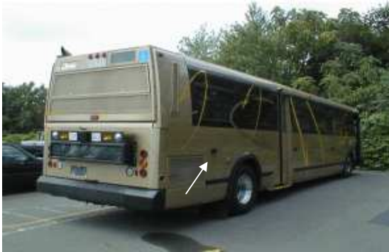
Figure 1 Transit bus with rear-looking and side collision warning systems (small black box, indicated by the arrow).
