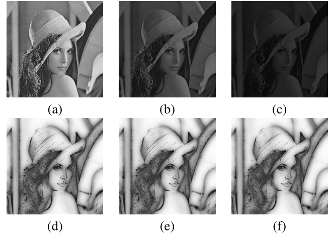
Fig. 4. IIFs. (a)–(c) Input images with different illuminations. (d)–(f) Corresponding outputs. These three results are obtained with the same \alpha .
