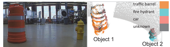
Fig. 6: The 3D classification: Both Object 1 (traffic barrel) and Object 2 (fire hydrant) are classified correctly with high confidence despite the fact that nearly a half of data points are mislabeled.
