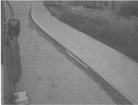
Fig. 3. Curb prediction: current detected curb location and future location found by image correlation
