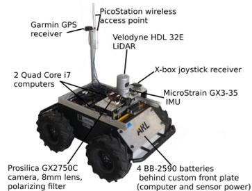
Fig. 7: Hardware configuration of the Clearpath Husky robot.
