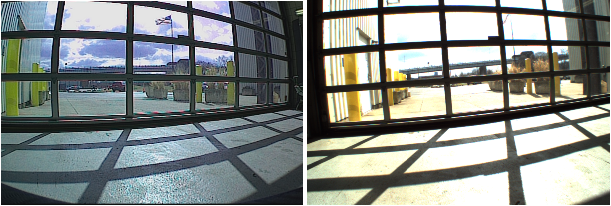
Figure 4. Left, sample image from Pixim SeaWolf captures detail in all regions, as compared to the Basler ACE camera, right. In particular, compare the floor where the shadows from the garage door are cast.
