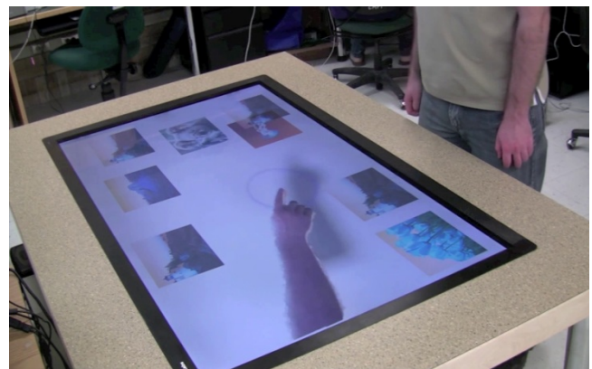
Figure 1: KinectArms used in a photo-sharing application, showing shadow and height indicator (circle).
