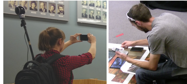
Figure 1. The 360° camera (atop a monopod affixed to a backpack) streams 360° video (left) to a tablet (right).
