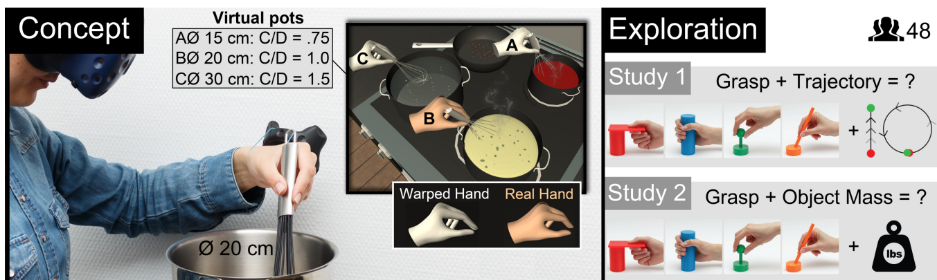
Figure 1: A user moves a proxy whisk inside a proxy pot (left). By offsetting the virtual hand/tool from the real hand/tool we can simulate virtual pots of different sizes providing realistic haptic sensations when stirring. Our studies investigate the extent to which we can use such illusions by exploring the potential effects of grasp, movement trajectory and object mass on the discrepancy which can be introduced while remaining unnoticed by a user.
