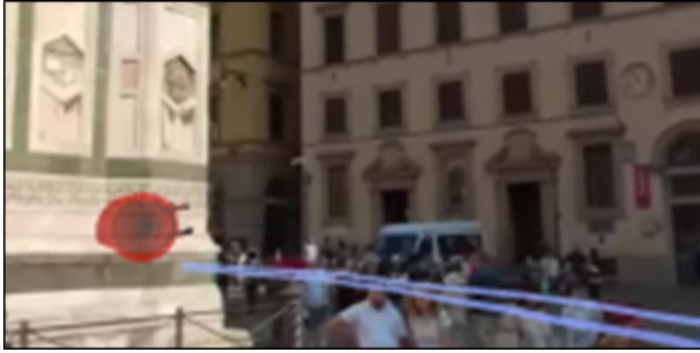
Fig. 7. A collaborator's avatar is rendered as a silhouette if they would normally be occluded by the environment (here, by the wall of the building).
