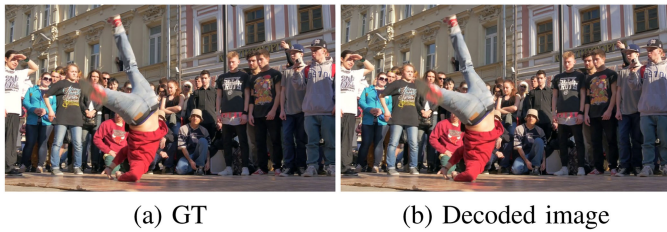
Fig. 6. Demonstration of the decoded image output by the decoder. Here, we only select one frame from the output sequence for a simple illustration. The difference between the groundtruth image (a) and decoded image (b) is visually imperceptible. The SSIM and PSNR values between (a) and (b) are: SSIM:0.9933 PSNR:40.166.
