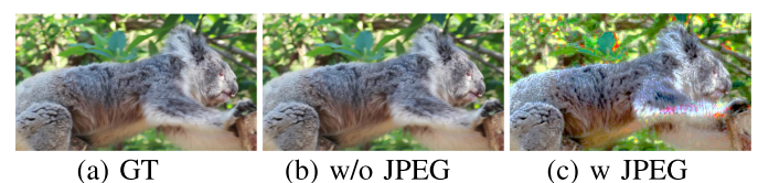
Fig. 18. Demonstration of the decoded image via JPEG compression. Here, we only select one frame from the sequence for a simple illustration. The visual difference between groundtruth image (a) and decoded without compression image (b) is imperceptible. But manifest visual difference observed with JPEG compression.
