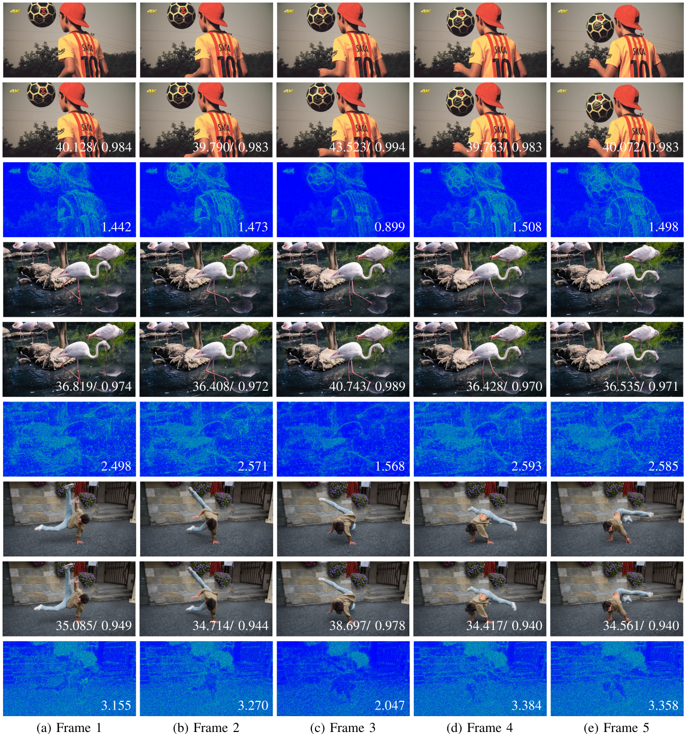
Fig. 13. Result gallery of the restored frames from the decoder. (a) to (e) contain of the complete input frames of the video. For each scene, images in the first row to the third row are the groundtruth frames, restored frames and the difference maps. PSNR, SSIM and MAE value are shown at the bottom right corner of corresponding images.
