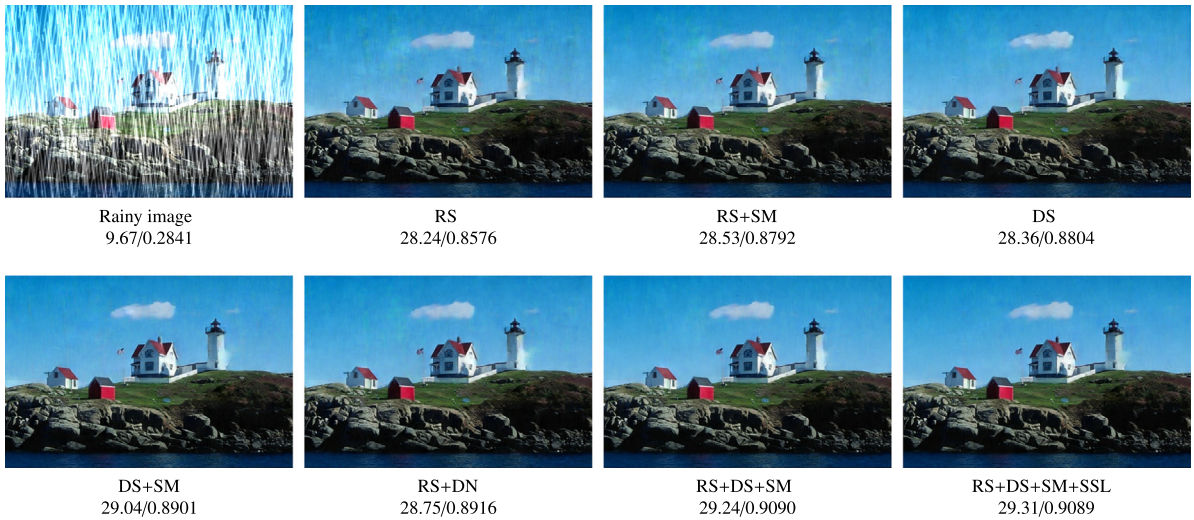
Fig. 3. Visual comparisons on Rain200H of different models in ablation study. PSNR/SSIM are listed below the images.
