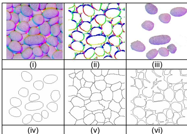
Figure 6. (i) Beach pebbles illuminated with RGB lights (ii) Edge map computed using multi-colour active illumination (iii) Manual identification of non-occluded particles using Photoshop (iv) Automatic identification of non-occluded particles (v) Edge map computed using marker-controlled watershed transform (vi) Edge map computed using canny edge detection
