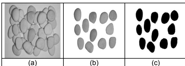
Figure 2. (a) Top view of overlapping particles (b) Manual identification of non-occluded particles (c) Automatic identification of non-occluded particles
