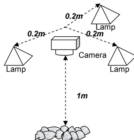
Figure 5. Hardware setup of camera with different illuminations
