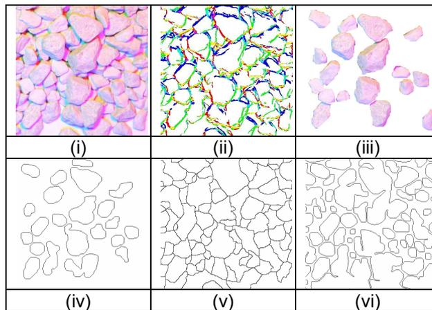
Figure 7. (i) Limestone illuminated with RGB lights (ii) Edge map computed using multi-colour active illumination (iii) Manual identification of non-occluded particles using Photoshop (iv) Automatic identification of non-occluded particles (v) Edge map computed using marker-controlled watershed transform (vi) Edge map computed using canny edge detection
