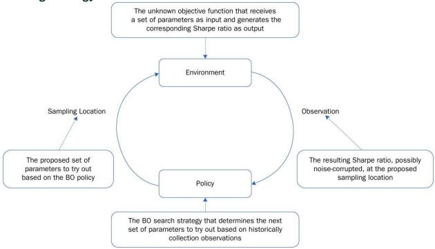
BO balances exploration and exploitation using two components: a GP to approximate the unknown objective function and an acquisition function that incorporates the exploration–exploitation tradeoff into a scalar value that reflects
