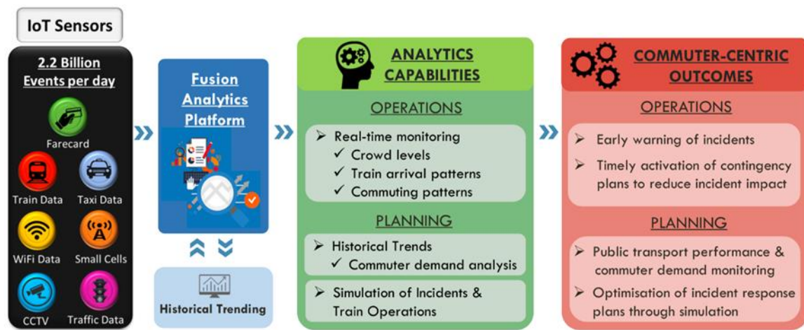
Figure 5: Summary of the FASTER system for predicting and responding to urban rail system disturbances and crowded commuter conditions. Source: Land Transport Authority of Singapore.
