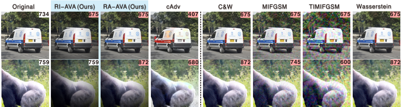
Figure 5: Adversarial examples generated with different methods. The top right corner shows the predictive label index and the ‘red’ numbers presents the attack misleads the DNN successfully. RI-AVA, RA-AVA, and cAdv are non-noise-based adversarial attack.
