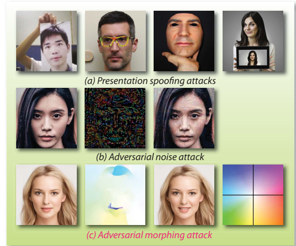
Figure 1: Three typical attacks on the FR systems. (a) presentation spoofing attacks (e.g., print attack [14], disguise attack [50], mask attack [36], and replay attack [8]), (b) adversarial noise attack [14, 18, 42], (c) proposed Amora.
