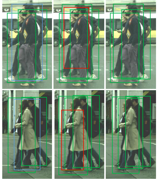
Fig. 5: Illustrative examples for different NMS algorithm. There are three pedestrians in each picture. The first column is the result of greedy-NMS, the mid column is density-aware NMS, and the last column is our attribute-aware NMS algorithm. The missed bounding box is colored by blue, and the false positive is denoted as red. There are three pedestrians in each picture, greedy
