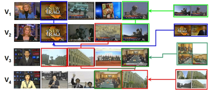
Fig. 2. TFIDF weighting of keyframe-based visual words. Within the 4 videos, four NDI clusters are shown and colored differently. For the red NDI cluster, it appears in V_2, V_3, V_4 , hence its df=3 , tf=2 for V_3 , tf=1 for V_2, V_4 . All non-NDI in a video have df=1 and tf=1 . Best viewed in color.
