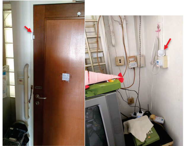
Fig. 4: Actual deployment of door contact sensor (left, red arrow) and living room PIR motion sensor (right, red arrow) in the SHINESeniors project
