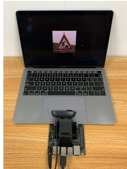
Fig. 6. Hardware setup to measure the execution time of the nine inference tasks (the photo was for the traffic sign recognition task, i.e. , the GTSRB dataset [43]) on the Jetson Nano embedded platform.
