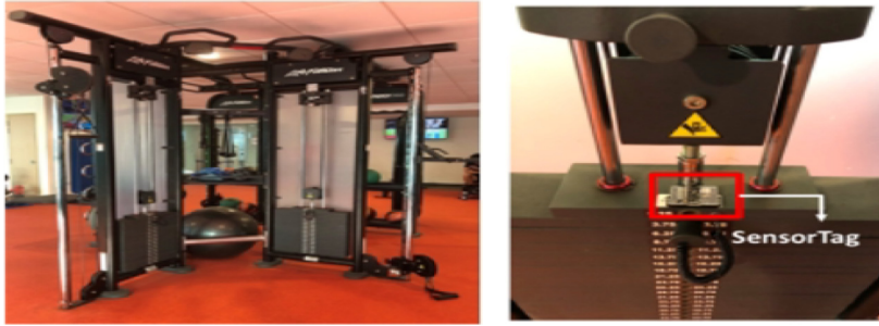
Fig. 1. Multi-purpose cable pulley machine and proposed sensor placement on the weight stack.
