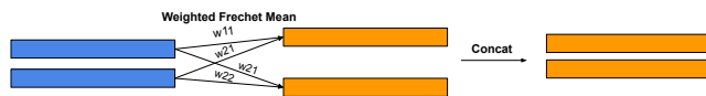
Figure 3: Weighted Riemannian Pooling: Performs multiple weighted Fréchet means on the channels of the input SPD
