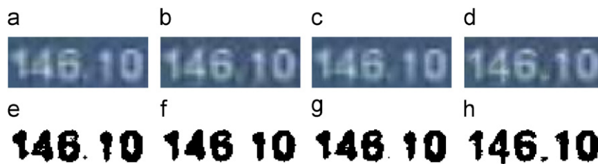
Fig. 7. Comparison between our approach and the algorithm proposed in Ref. [36]. (a) and (b) are two text boxes in low resolution, (c) is the averaged textbox by the algorithm in Ref. [36]. (d) is the high-resolution textbox reconstructed by our approach. (e)–(h) are the binarized textboxes of (a)–(d).
