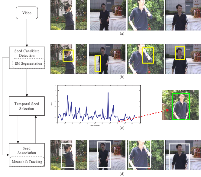
Fig. 1. Proposed framework. (a) Four sample video frames in a shot; (b) The bag of detected candidates indicated by the bounding boxes in the sample frames; (c) The first seed (right) is selected based on the computed saliency plot (left) with y-axis shows the fidelity of seed candidates in the shot; (d) The result of extracting objects after propagating and associating the first seed in (c) with the candidates at (b).
