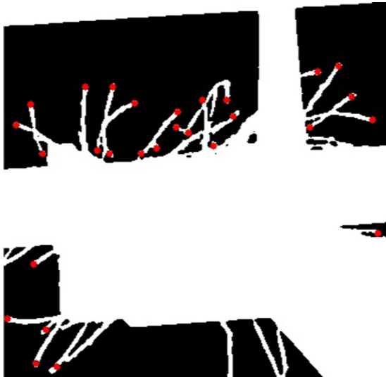
Fig. 7. Detected hovering points of a bird nest candidate, which are labeled in red dots. (For interpretation of the references to color in this figure legend, the reader is referred to the web version of this article.)
