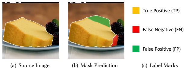
Figure 7: Calculating IoU and Acc, taking the “cake” mask as an example. \text{IoU} = \frac{\text{TP}}{\text{TP}+\text{FP}+\text{FN}} and \text{Acc} = \frac{\text{TP}}{\text{TP}+\text{FN}} .
