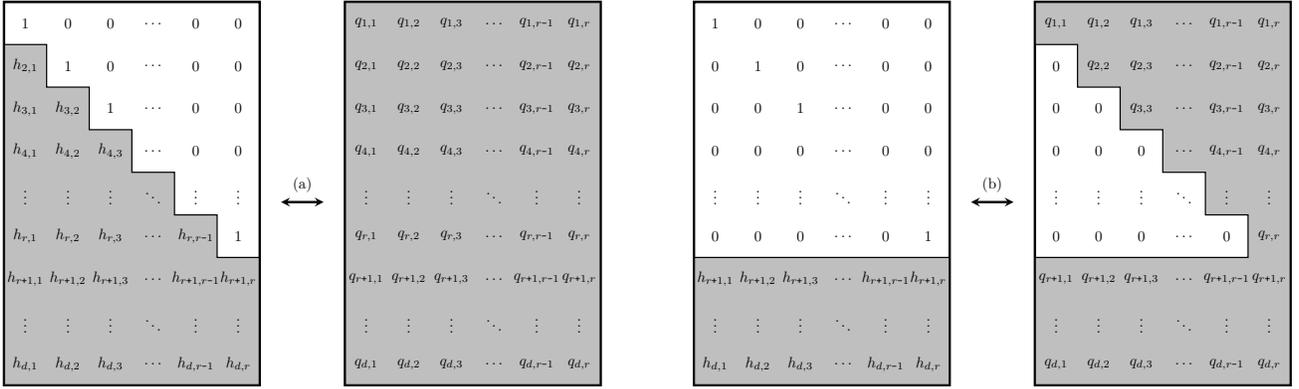
Figure 3: Visualization of Householder parameterizations of orthonormal frames as per the LAPACK convention: (a) Full parameterization, (b) Reduced parameterization. Shaded areas with  $h_{i,j}$  values represent parameters of reflectors;  $q_{i,j}$  values represent orthonormal frame elements, affected by the corresponding parameterization.
