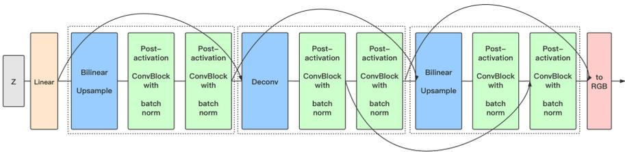
**Fig. 3.** The generator architecture discovered by E<sup>2</sup>GAN on CIFAR-10.
