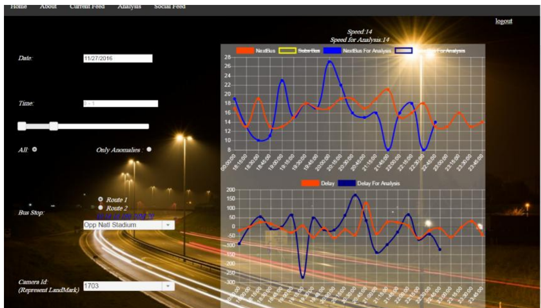
Figure 5: The Analytics Dashboard Depicting the Next Bus Arrival Times Super-Imposed with the Expected Arrival Times for Bus Service No. 16 at the Bus Stop Opposite of the National Stadium.
