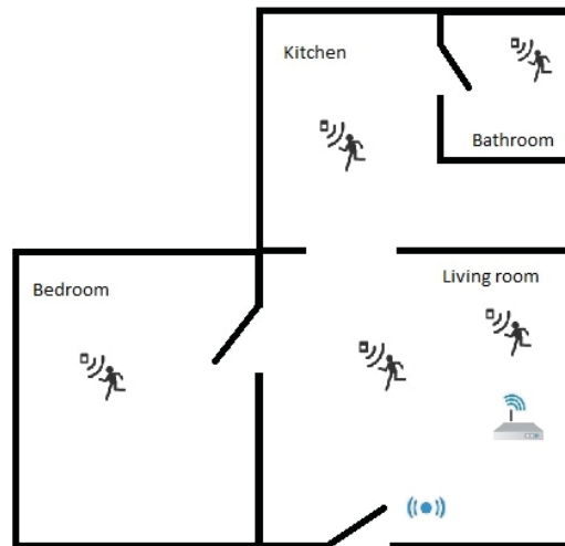
Figure 3 Sensor deployment in Bedok in a 2-room flat
