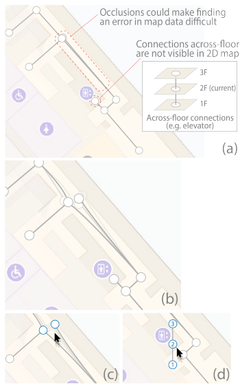
Figure 1: (a) Node/edge occlusions and across-floor connections make it difficult to find topological errors when a map for a multi-floor building was manually composed. (b) We design a technique that visualizes these occluded elements with micro-animation ( repel ) to support users to find them. We also design an interaction technique that visualizes (c) occlusions and (d) across-floor connection relationships related to the element near the cursor, which supports users acquire and edit the occluded elements.
