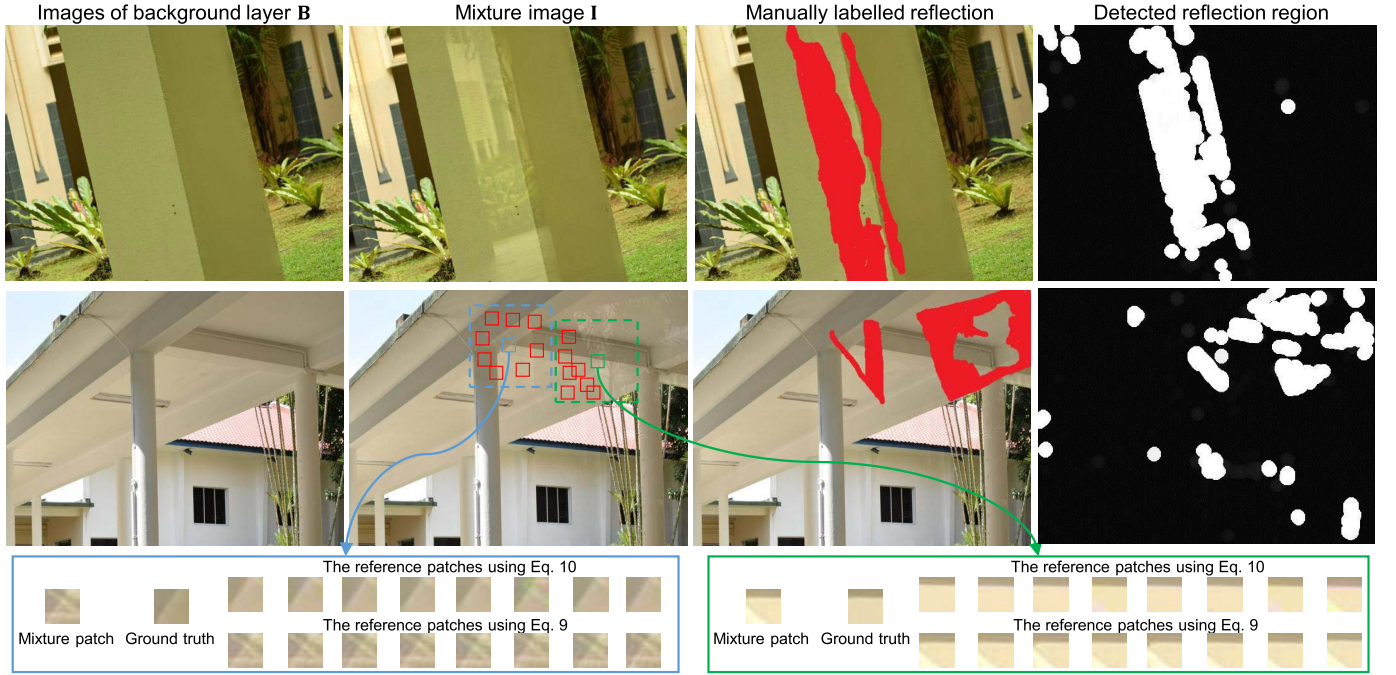
Fig. 3. Two examples of the detected reflection dominant regions (white pixels in the rightmost column) with their corresponding images of background, mixture images, and reference of reflections identified by humans (red pixels in the third column). At the bottom row, we show two examples of the patch matching results (the patch brightness \times 2 for better visualization). Given the mixture patch with reflections, we show its corresponding ground truth without reflections (extracted from \mathbf{B} ) and the reference patches found using Equation (9) and Equation (10) (extracted from \mathbf{I} , with dashed box as the searching window), respectively. The reference patches found using Equation (10) are more similar to ground truth than the patches found using Equation (9).
