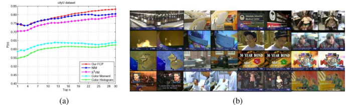
Fig. 8. (a) Top- n IND retrieval performance of FCP and relevant methods on the CityU's TRECVID2004 dataset. (b) Examples of IND pairs returned by the proposed FCP where scale, illumination, viewpoint, as well as image editing changes occur.
