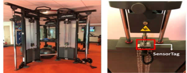
Fig. 1: Multi-Purpose Cable Pulley Machine and Proposed Sensor Placement on the Weight Stack
