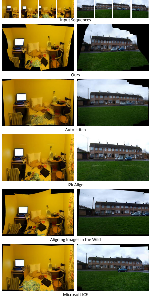
Figure 8. Mosaics creating by panning a camera in the X -direction. The results are shown for Ours, Auto-Stitch [5], I2K [1], Aligning Images in the Wild [21] and Microsoft ICE [27]
