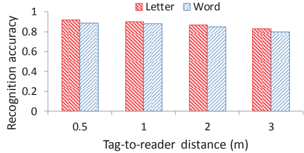
Figure 24— Impact of tag-to-reader distance.
