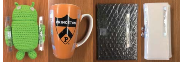
Figure 25— Making a stylus using everyday object.
