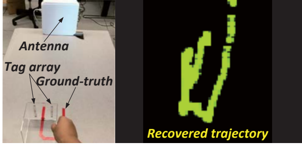
Figure 12 — Recovering the trajectory of the moving cube based on pseudo-ranging.
