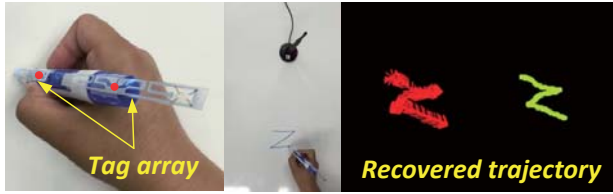
Figure 2— Handwriting tracking: the antenna is placed near the pen for a better illustration. Tag spacing = 2.7cm.
