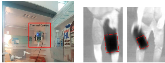
(a) Camera setup inside the fridge (b) Sample thermal images taken by thermal camera
