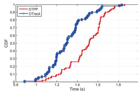
Figure 23: Ordering latency of STPP and OTrack
