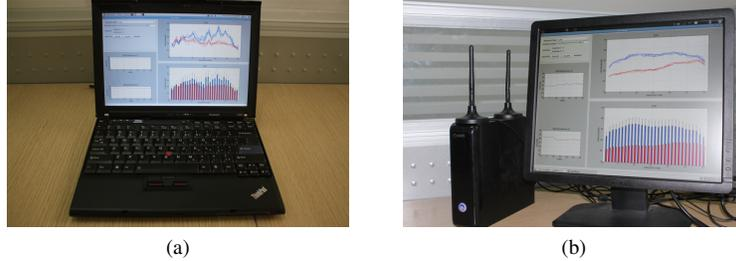
Fig. 9. Receiver setup: (a) a laptop equipped with internal Intel 5300 NIC; (b) a mini PC with external Intel 5300 NIC.
