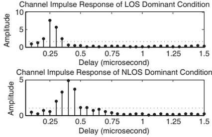
Fig. 2. Sampled version of CIR derived from CSI.
