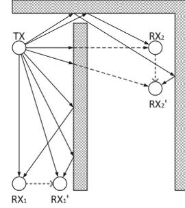
Fig. 5. Impact of mobility on LOS/NLOS propagation.
