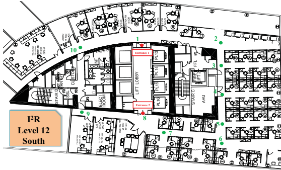
Fig. 3. Testbed - I 2 R Level 12 South. It contains both straight and curved corridors. The two entrances are labeled in red. The green dots are the waypoints for ground truth collection.
