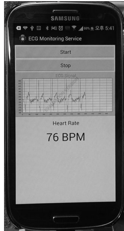
Fig. 4. A screenshot of the example healthcare application. The application shows the electrocardiogram (ECG) waveform and heart rate of the user in real time. BPM, beats/min.
