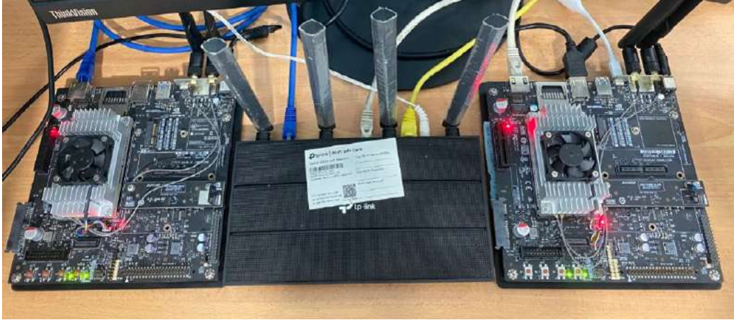
Figure 4.5: JIGSAW 's System Test Bed with 2x NVIDIA Jetson TX2 device (primary/secondary)
