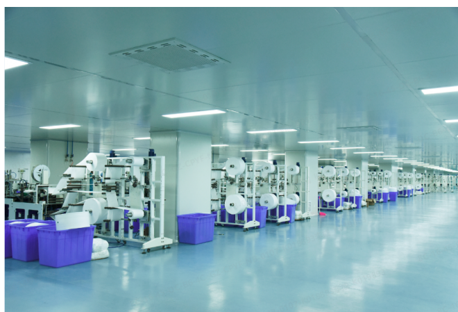
Figure 1-3 Class 100,000 Cleaning Workshop
