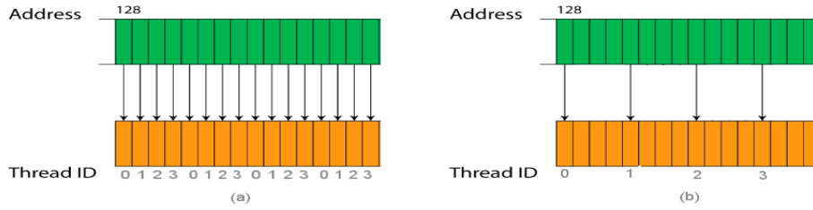
Figure 2.5: Memory Coalescing vs Memory Vectorization
